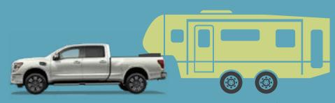
TITAN XD up to 11,000 lbs6 Integrated gooseneck hitch connects in the truck bed
